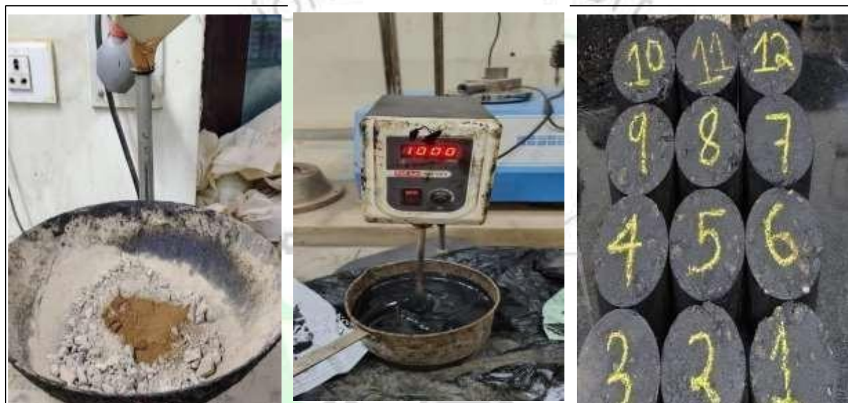
Figure 4(a) : Marshall mix design using dry and wet method
