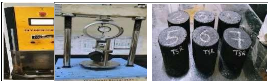
Figure 4(b): ITS and TSR testing procedure
